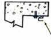
Door guide installed behind the opening.
